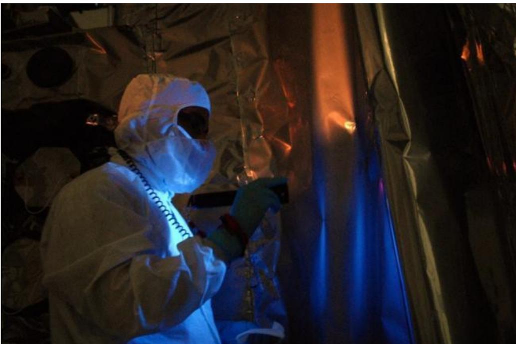
Figure 2: Black light contamination inspection for the Lunar Reconnaissance Orbiter (LRO)<sup>3</sup>.
